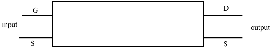
Figure 5.17 Two-port representation of the small signal model of a JFET. The inputs are the gate and source while the outputs are the drain and source as shown in the diagram.
